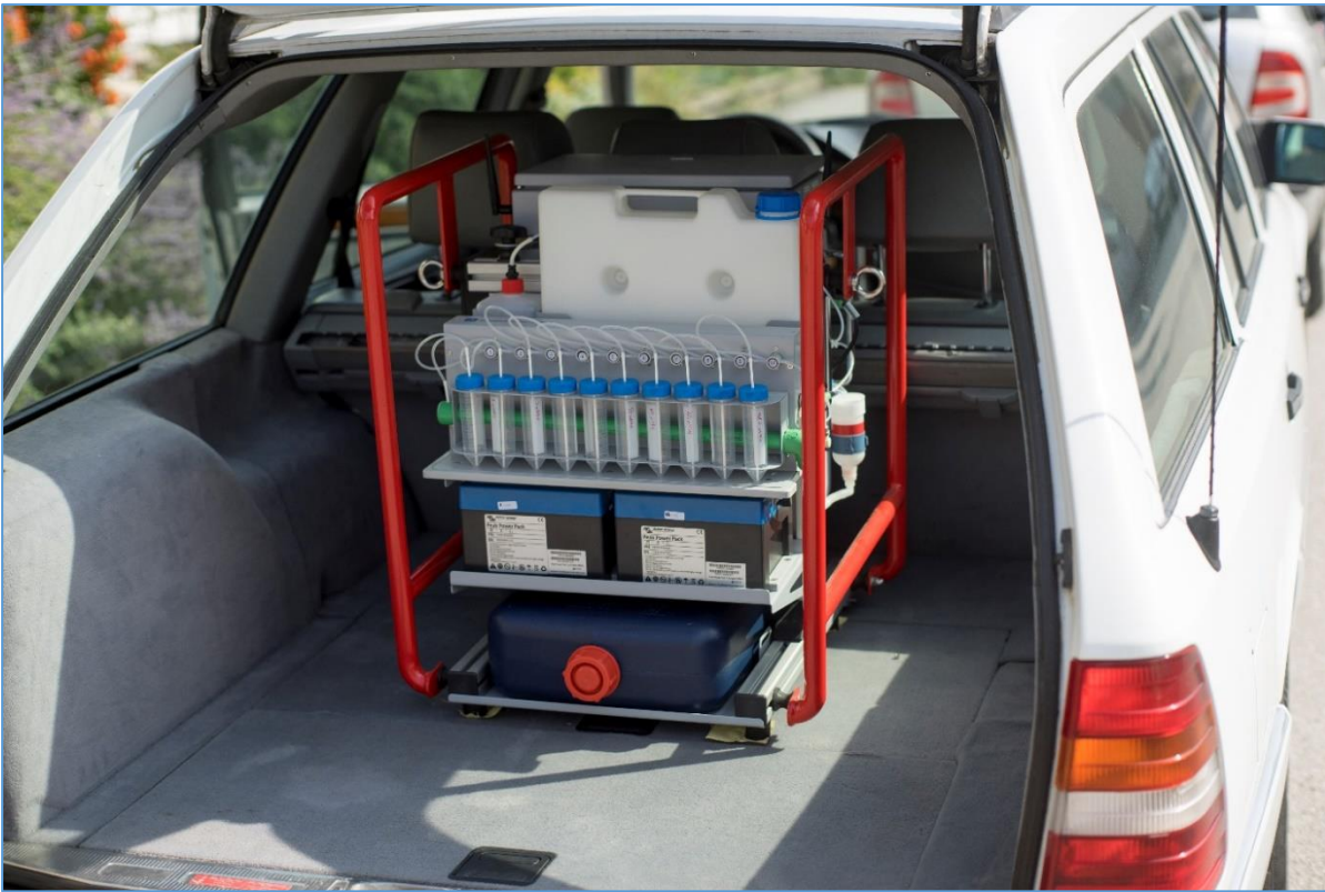
FIGURE 1: ERU (COLIMINDER EMERGENCY RESPONSE UNIT) IN A CAR
